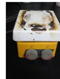
Where only stirring is required, acquire and use a stirrer instead of a hotplate/stirrer combination.
