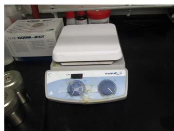
Older hotplates with relay heater switches can spontaneously heat in the heater dial OFF position
