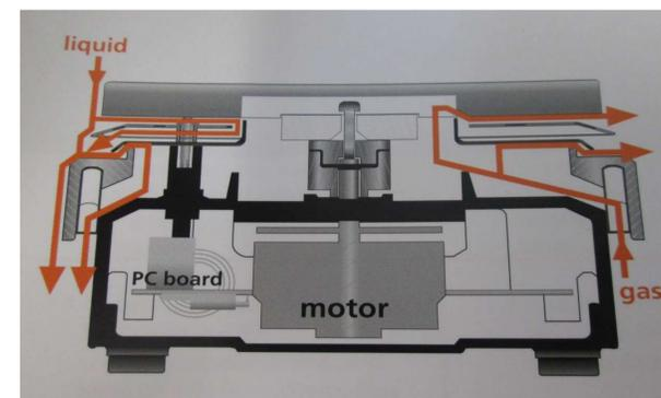
Additional hotplate safety features to look for are two independent temperature control circuits, which switch off heating in case of an over temperature situation.
