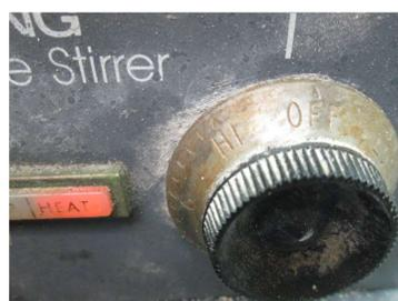
Liquids in contact with electronics may cause shorts. Newer hotplates with TRIAC or microprocessor-controlled heater switches may spontaneously heat in the OFF position due to liquid exposure to the electronics
