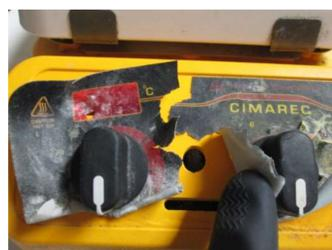
Potential for liquid access through front cover and/or slots in housing.
