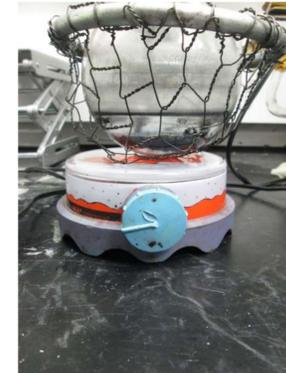
Unplug inactive hotplates or heating mantles in close proximity to oil baths, combustible or flammables material.
